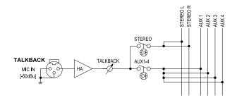
Use the talkback function to send instructions mainly from the operator to musicians and studio staff. This section adjusts the level of the microphone signal received from the TALKBACK MIC IN jack, and determines the bus to be output.
