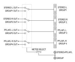
Use these meters to view various signal levels: the levels to the STEREO OUT L/R jacks, the PFL and AFL levels, and the levels to the GROUP OUT 1-4 jacks. The PFL or AFL signals indicated by these meters can be monitored through the MONITOR OUT jacks and the PHONES jack.
