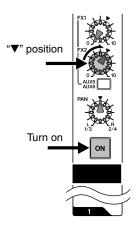
5. Rotate the FX TO FX BLEND knob fully counter-clockwise.
