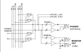
You connect a pair of headphones and adjust the output signal level to the PHONES and MONITOR OUT jacks.
