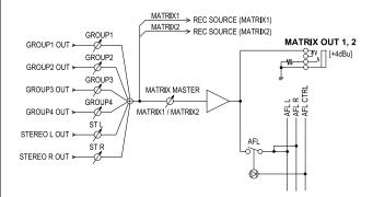
This section adjusts the levels and controls the output of signals to the MATRIX OUT jacks from GROUP OUT and STEREO OUT. The signals from the MATRIX 1 and 2 buses are sent to the MATRIX 1 and 2 jacks respectively.
