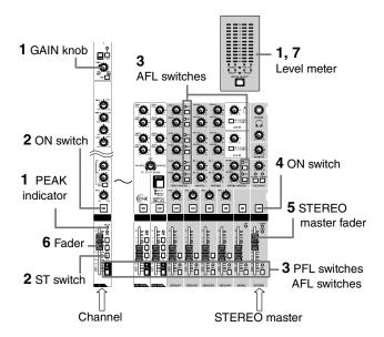
While producing sound on your instrument or microphone, adjust the channel GAIN knobs so that the corresponding peak indicators flash briefly at the highest peak levels.
