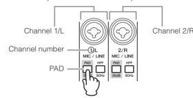
NOTE If you are using condenser microphones, turn on (♠) the [PHANTOM +48V] switch.
