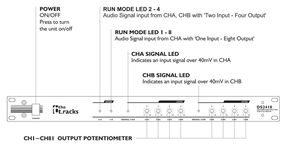
Turn these potiknobs clockwise to gradually increase the signal output up to +6dB. Turn these potiknobs counter-clockwise to gradually decrease the signal output down to nil.
