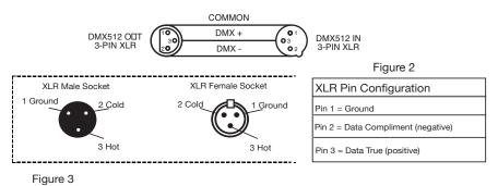
**Special Note: Line Termination.** When longer runs of cable are used, you may need to use a terminator on the last unit to avoid erratic behavior. A terminator is a 110-120 ohm 1/4 watt resistor which is connected between pins 2 and 3 of a male XLR connector (DATA + and DATA -). This unit is inserted in the female XLR connector of the last unit in your daisy chain to terminate the line. Using a cable terminator (ADJ part number Z-DMX/T) will decrease the possibilities of erratic behavior.
